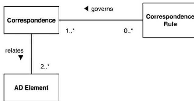
NOTE The figure uses the conventions for class diagrams defined in [ISO/IEC 19501].
