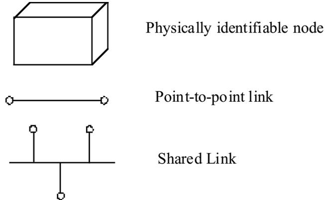
One diagram is provided for each identified communication layer. Each diagram is annotated to show the addressing, link access, and routing/switching strategies at each link.
